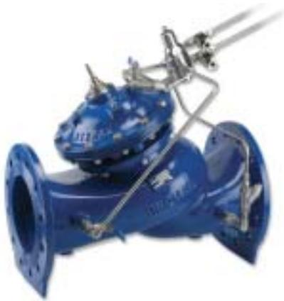
The Model 736-ES-VI Differential-Pressure Sustaining Valve is a hydraulically-operated, diaphragm-actuated, control valve that sustains minimum pre-set, differential pressure between two points regardless of fluctuating flow or varying upstream pressure.
