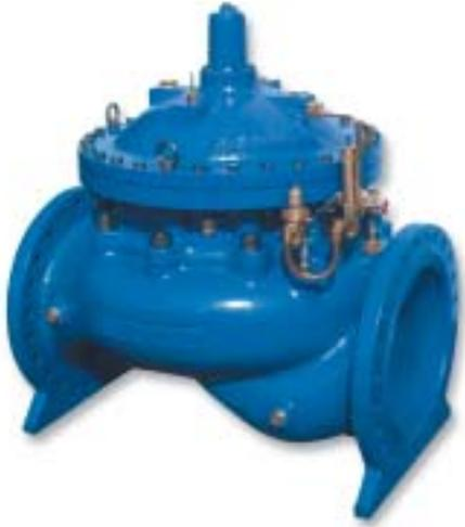
BERMAD DN 600, DN 700, DN 750 & DN 800 700 Series Control Valves are hydraulically operated, diaphragm actuated globe pattern valves. The valve is comprised of two major components, the body assembly and the actuator assembly. The actuator assembly is removable from the body as an integral unit. It consists of two control chambers, an upper and a lower. The actuator can be converted on-site from single to double-chambered actuator and vice-versa according to the required control function.
