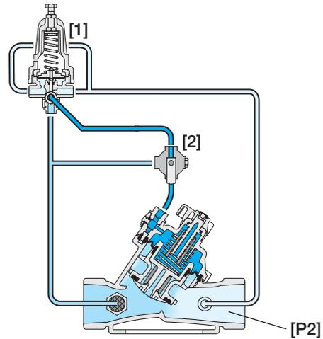
The Pressure Reducing Servo Pilot [1] commands the main Valve to throttle closed, preventing Downstream Pressure [P2] from rising above pilot setting, and to modulate open when [P2] drops below pilot setting. The Manual Selector [2] enables local manual closing.
