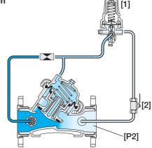
The Pressure Reducing Pilot [1] commands the Valve to throttle closed should Downstream Pressure [P2] rise above setting, and modulate to open when it drops below setting. The downstream Cock Valve [2] enables manual closing.
