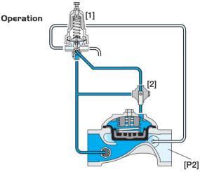
The Pressure Reducing Pilot [1] commands the main Valve to throttle closed should Downstream Pressure [P2] rise above pilot setting and to open fully when it drops below pilot setting. The Manual Selector [2] enables local manual closing.
