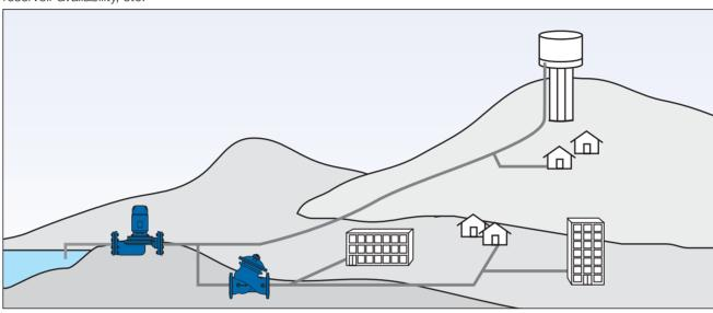
The pump supplies water to the network and to the reservoir. System pressure is too high for the residential neighborhood, requiring a pressure reducing system.
