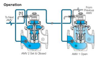
Each AMV is manually preset to deliver a desired quantity of water. Pressure from the previous AMV enters the current AMV control chamber through its Sequential Shut-Off Pilot (SSOP) [1], closing it. The current AMV inlet pressure is transmitted to the Next AMV, closing it. When the previous AMV shuts itself, it allows the current AMV control chamber to drain through both the current and Previous AMV's SSOP's, opening the current AMV. The next AMV remains closed until AMV-2 shuts itself.
