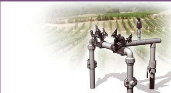
Located at the entrance to the distribution lines and laterals, the Infield Head-Works serves as the system's final control. Including a range of multi-features remote control valves, governed by the irrigation controller, the Infield Head-Works Controls irrigation shifts, applies water metering abilities, maintains pre-designed system flow & pressure, establishes pressure zones to protect the laterals, Incorporates local fertilization arrangements and final filtration solutions.
