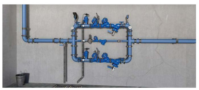
Two-Stage Pressure Reducing Station, featuring BERMAD BC-720-PD-P valves to reduce the incoming pressure by a fixed ratio and share the load with the BERMAD BC-720-P PRV, a redundant, parallel branch to minimize the possibility of total water shut-off and a low flow bypass branch for low demand operation. For information on the other BERMAD products in this system please see the product data sheet for the following components: BERMAD BC-720-P, BERMAD BC-73Q-P and BERMAD BC-70F-P.
