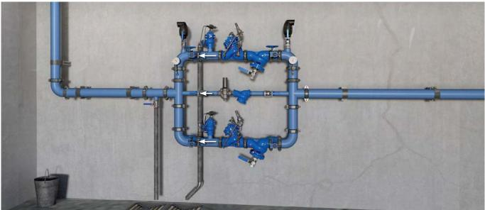
Pressure Reducing Station, featuring BERMAD BC-720-P valves to reduce high incoming pressure to a lower downstream set-point, a redundant, parallel branch to minimize the possibility of total water shut-off and a low flow bypass branch for low demand operation. For information on the other BERMAD products in this system please see the product data sheet for the BERMAD BC-73Q-P and BERMAD BC-70F-P.
