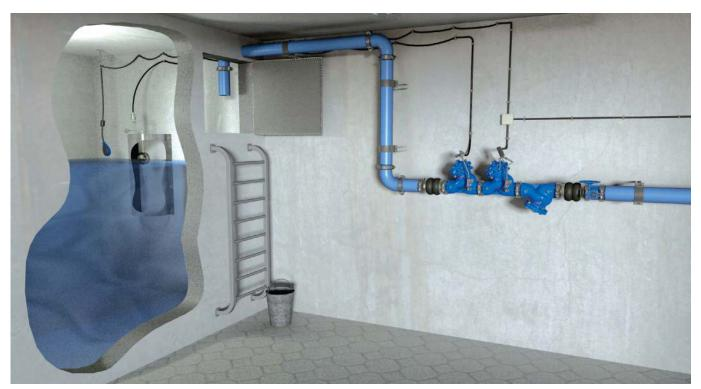
Water Reservoir Level Control System, featuring the BC-750-67-P that maintains constant water level in the reservoir. As backup another level control valve is stationed upstream and calibrated to a slightly higher water level. The backup valve can be specified to operated hydraulically (BC-750-66-P) or electrically (BC-750-65-P).
