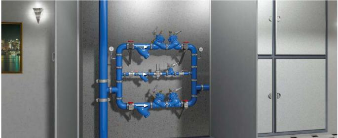
Pressure Reducing Station, featuring BERMAD BC-794-P valves to prevent high pressure from reaching consumers, a redundant, parallel branch to minimize the possibility of total water shut-off and a low flow bypass branch for low demand operation. For information on the other BERMAD products in this system please see the product data sheet for the BERMAD BC-720-P and BERMAD BC-70F-P.
