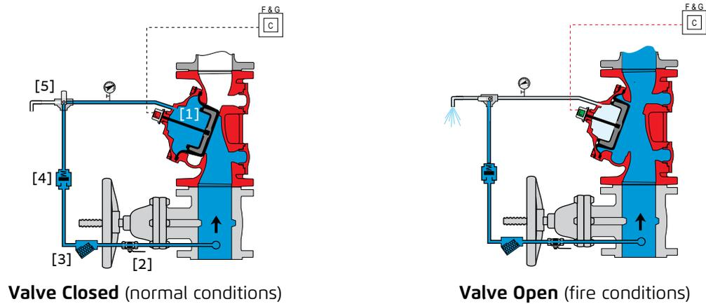
The BERMAD model 400Y-11 is held closed by water pressure in the control chamber [1]. Upon release of pressure from the control chamber, the valve opens.
