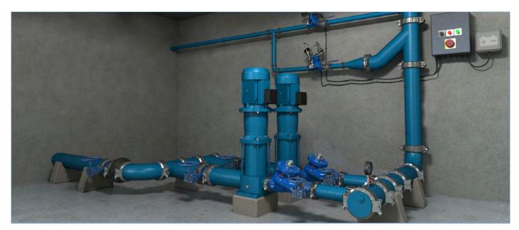
Lift Pump Station with BERMAD Check Valve preventing reverse flow into the reservoir. The station also features a BC-730-P Pressure Relief Valve that maintains minimal flow if churn operation occurs, and BC-
