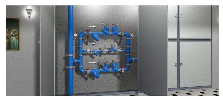
**Pressure Reducing Station**, featuring BERMAD BC-794-P valves to prevent high pressure from reaching consumers, a redundant, parallel branch to minimize the possibility of total water shut-off
