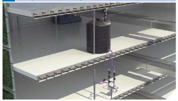
Teated Recycled water for sanitation use - using cooling towers water for toilet flushing, floors washing and irrigation.
