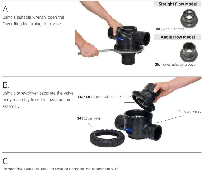
Inspect the seats visually. In case of damage, go tonext step (C).
