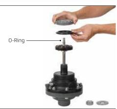
Replace the components of the closure assembly in the order shown here, from bottom to top. Pay attention to the position of the parts and their direction according to the different models (Angular model - black cover; Straight model - gray cover).
