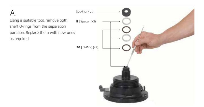
Use a silicon lubricant when reassembling the shaft.
