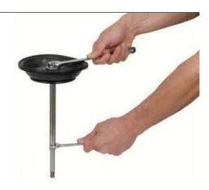
Remove the diaphragm washer. Check and replace diaphragm as required.
