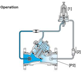
The Pressure Reducing Pilot [1] commands the Valve to throttle closed should Downstream Pressure [P2] rise above setting, and modulate to open when it drops below setting. The downstream Cock Valve [2] enables manual closing.
