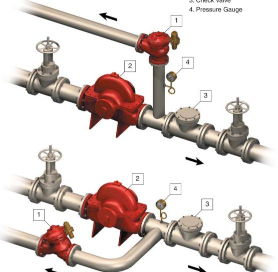
Installation with "Y" Pattern Pressure Relief Valve
