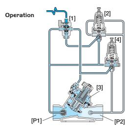
The 3-Way Hydraulic Relay Valve (3W-HRV) [1] hydraulically connects the Pressure Reducing Servo Pilot (PRSP) [2] to the Valve Control Chamber [3]. The PRSP commands the Valve to throttle closed, preventing Downstream Pressure [P2] from rising above pilot setting. The 3W-HRV switches upon pressure drop command, causing the main Valve to shut. Should Upstream Pressure [P1] rise above setting, the Relief Pilot [4] opens, thereby opening the Valve to relieve excessive pressure.
