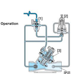
The 3-Way Hydraulic Relay Valve (3W-HRV) **[1]** hydraulically connects the Pressure Reducing Servo Pilot (PRSP) **[2]** to the Valve Control Chamber **[3]**. The PRSP commands the Valve to throttle closed, preventing Downstream Pressure **[P2]** from rising above pilot setting. The 3W-HRV switches upon pressure drop command, directing line pressure into the control chamber, and thereby causing the main Valve to shut. The 3W-HRV also features local manual closing.
