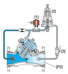
Opening the Solenoid [1] opens the Valve. The Pressure Reducing Pilot [2] commands the valve to throttle closed should Downstream Pressure [P2] rise above setting, and to modulate open when it drops below setting. Closing the solenoid causes the Valve to shut. The downstream Cock Valve [3] enables manual closing.
