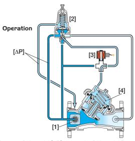
Pressure Differential [ $\Delta P$ ] across the Differential Pressure Duct [1] is in direct proportion to demand. The Flow Pilot [2] continuously senses [ $\Delta P$ ] and commands the Valve to throttle closed should demand rise above pilot setting. The Solenoid [3] hydraulically connects the flow pilot to the main Valve Control Chamber [4]. In response to an electric signal, the solenoid switches, directing line pressure into the control chamber and causing the main Valve to shut.
