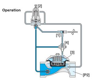
The Shuttle Valve [1] hydraulically connects the Pressure Reducing Servo Pilot (PRSP) [2] to the valve Control Chamber [3]. The PRSP commands the valve to throttle closed, preventing Downstream Pressure [P2] from rising above pilot setting. Upon pressure rise command, the shuttle valve automatically switches, allowing pressurization of the control chamber, which causes the main Valve to shut. The Manual Selector [4] enables manual closing.
