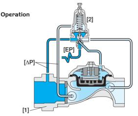
Pressure Differential  $[\Delta P]$  across the Orifice Assembly [1] is in direct proportion to backwash flow rate.
