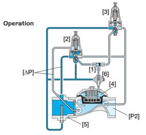
The Shuttle Valve [1] hydraulically connects the Flow Pilot (FP) [2] or the Pressure Reducing Pilot (PRP) [3] to the Valve Control Chamber [4]. Pressure Differential [ $\Delta P$ ] across the Orifice Assembly [5] is in direct proportion to demand. The FP, continuously sensing [ $\Delta P$ ], commands the Valve to throttle closed should demand rise above setting. The PRP commands the AMV to reduce Downstream Pressure [P2] to pilot setting. The Manual Selector [6] enables local Manual closing.
