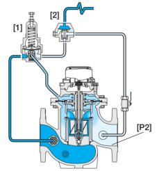
The Pressure Reducing Pilot [1] commands the Hydrometer to throttle closed should Downstream Pressure [P2] rise above setting, and to modulate open when it drops below setting. The 3-Way Hydraulic Relay Valve [2] opens upon receiving remote pressure rise command opening the Hydrometer, and closes in the absence of this command shutting the Hydrometer.
