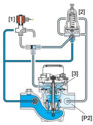
The Solenoid [1] hydraulically connects the Pressure Reducing Servo Pilot (PRSP) [2] to the Hydrometer Control Chamber [3]. The PRSP commands the Hydrometer to throttle closed, preventing Downstream Pressure [P2] from rising above pilot setting. In response to an electric signal, the solenoid switches, directing line pressure into the control chamber, and thereby causing the Hydrometer to shut. The Solenoid also features local manual closing.
