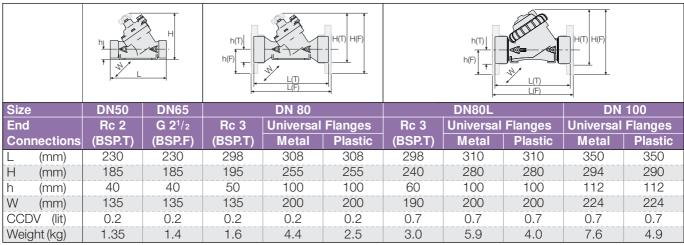
CCDV = Control Chamber Displacement Volume
