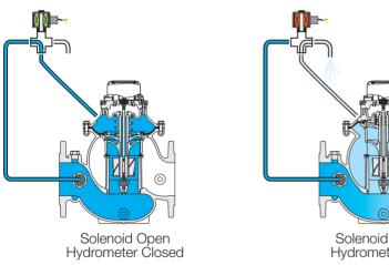
Solenoid Closed Hvdrometer Open
