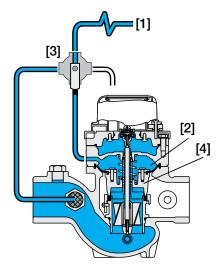
Hydraulic Command [1] is applied to the Control Chamber [2], through the Manual Selector [3]. This creates a superior closing force that moves the Diaphragm Assembly [4] to a closed position. Discharging pressure from the control chamber, by turning the manual selector, causes the line pressure acting on the lower side of the diaphragm assembly to move the Hydrometer to an open position, and measure the flow rate.
