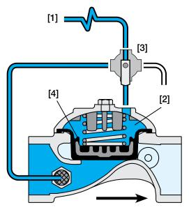
Hydraulic Command **[1]** is applied to the Control Chamber **[2]** through the Manual Selector **[3]**. This creates superior closing force that moves the Diaphragm Assembly **[4]** to a closed position. Discharging pressure from the control chamber, by turning the manual selector, causes the line pressure acting on the lower side of the diaphragm assembly to move the Valve to an open position.
