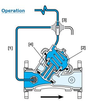
Line Pressure [1] is applied to the Control Chamber [2] through the Manual Selector [3]. This creates superior closing force that moves the Diaphragm Assembly [4] toward a closed position. The discharge of pressure from the control chamber causes the line pressure acting on the diaphragm assembly to move the valve to an open
