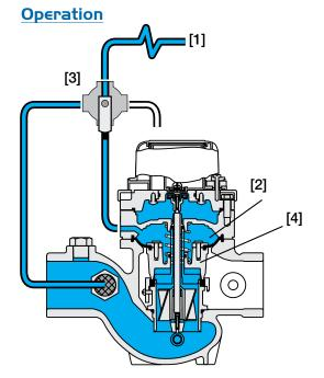
A Hydraulic Command [1] is applied to the Control Chamber [2], through the Manual Selector [3]. This creates a superior closing force that moves the Diaphragm Assembly [4] to a closed position. Discharging pressure from the control chamber, by turning the manual selector, causes the line pressure acting on the lower side of the diaphragm assembly to move the Hydrometer to an open position, and measure the flow rate.
