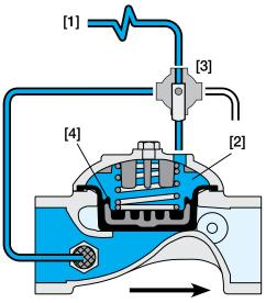
Hydraulic Command [1] is applied to the Control Chamber [2] through the Manual Selector [3]. This creates superior closing force that moves the
