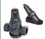
Adjustable Direct Acting Pressure Reducers with rolling diaphragm that Isolates mechanism from flow & minimizes friction, providing accurate reliable control.
