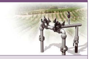
Located at the entrance to the distribution lines and laterals, the Infield Head-Works serves as the system's final control. Including a range of multi-features remote control valves, governed by the irrigation controller, the Infield Head-Works Controls irrigation shifts, applies water metering abilities, maintains pre-designed system flow & pressure, establishes pressure zones to protect the laterals, Incorporates local fertilization arrangements and final filtration solutions.
