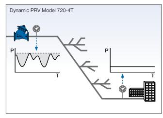
The dynamic PRV - Model 720-4T, integrated with a PR controller, is designed to continuously correct its set value based on the momentary demand and/or minimum required pressure at the system critical point.
