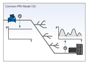
Common PRVs are set to maintain a constant low downstream pressure, ensuring sufficient pressure at the system's critical point during peak demand (when line friction head loss is highest). The shaded area represents the hours and levels when pressure is higher than required.
