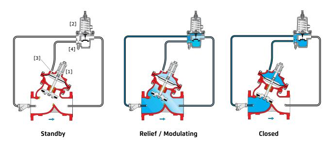
**Standby:** The BERMAD 730-48 is a Normally Open valve with an external lifting spring [1] keeping the valve in a fully open position as default when the system piping is depressurized, as might be before a pump start-up. When the pump starts the initial pressure surge and excess air will be expelled from the system through the valve.
