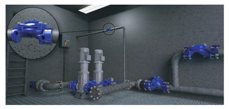
The BERMAD 430 As a pressure sustaining valve that recycles water back to the reservoir at stagnate pump operation, it will remain close when raiser pressure is normal. In an event where the pump works at low flows and high head, the 430 will open to allow sufficient water
