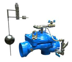
Water Reservoir Level Control System, featuring the 450-67 that maintains constant water level in the reservoir. As backup another level control valve is stationed upstream and calibrated to a slightly higher water level. The backup valve can be specified to operated hydraulically (450-66) or electrically (450-65).
