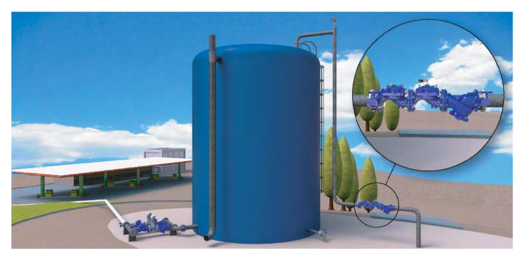
BERMAD 450-80 maintains high and low water levels with high accuracy pilot valve that senses reservoir water level head from a sensing point at the bottom of the reservoir and controls the main filling valve
