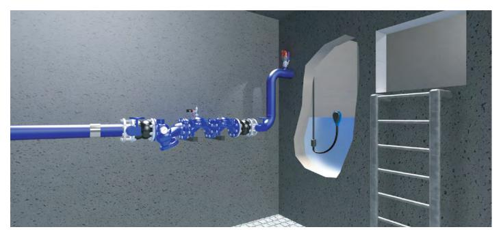
Water Reservoir Level Control System, featuring the 453-65 as an electric controlled backup valve to an hydraulically controlled level control valve. In case of main level control valve malfunction the Electric Float will sense the rise in water level and signal the 453-65
