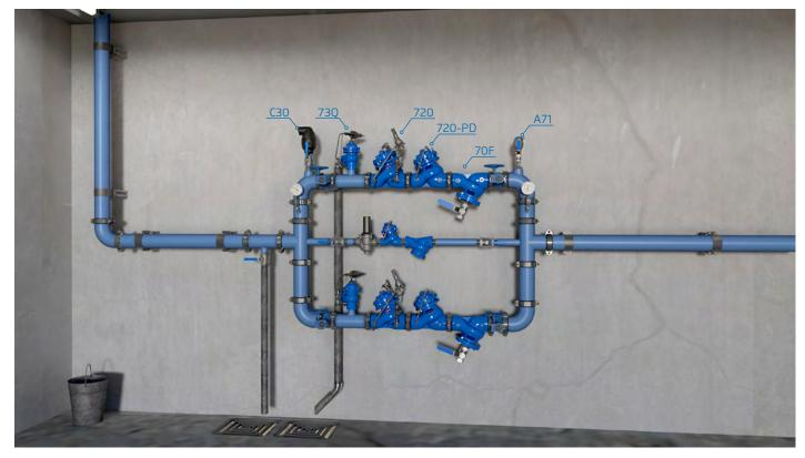
Two-Stage Pressure Reducing Station, featuring BERMAD 720-PD valves to reduce the incoming pressure by a fixed ratio and share the load with the BERMAD 720 Pressure Reducing Valve, a redundant, parallel branch to minimize the possibility of total water shut-off
