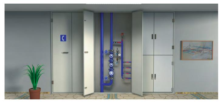
Pressure Reducing System, featuring a BERMAD 72S-2B-H system to reduce high incoming pressure to a lower downstream setpoint while minimizing the possibility of total water shut-off with integrated low flow bypass branch for low demand operation. For information on the other BERMAD products in this system please see the product data sheet for the BERMAD 73Q and BERMAD 70F.
