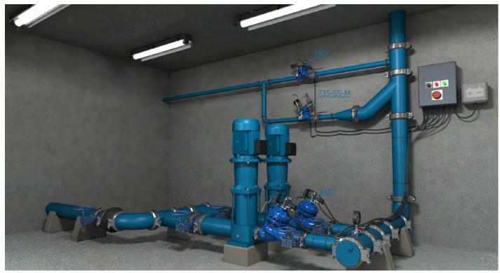
The BERMAD 730 As a pressure sustaining valve that recycles water back to the reservoir at stagnate pump operation, it will remain close when raiser pressure is normal. In an event where the pump works at low flows and high head, the 730 will open to allow sufficient water circulation and pump cooling. Also featured is the 740 Active-
