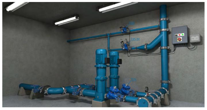
A soft start/stop pump station with emergency surge protection - in a case of power failure sudden pressure drop due to column separation will activate the 735-M to open and anticipate any returning surge from the riser, thus reducing water hammer damage and prolonging equipment lifetime.
