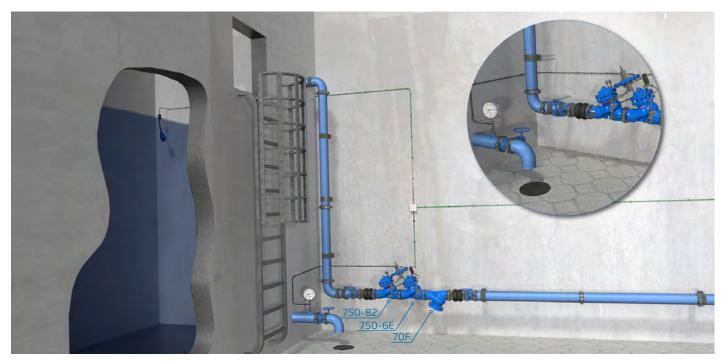
With BERMAD 750-82 the water level is maintained by the use of a highly accurate pilot valve that precisely senses the water level head from a sensing point at the bottom of the reservoir and controls the
