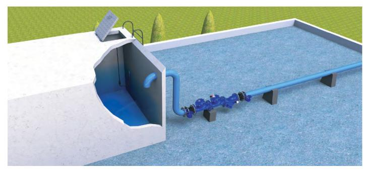
Water Reservoir Level Control System, featuring the 753-65 as an electric controlled backup valve to an hydraulically controlled level control valve. In case of main level control valve malfunction the Electric Float will sense the rise in water level and signal the 753-65
