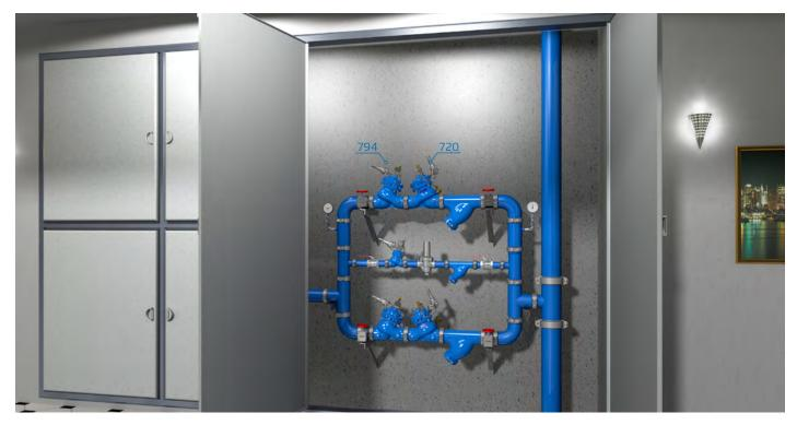
Pressure Reducing Station, featuring BERMAD 794 valves to prevent high pressure from reaching consumers, a redundant, parallel branch to minimize the possibility of total water shut-off and a low flow bypass branch for low demand operation. For information on the other BERMAD products in this system please see the product data sheet for the BERMAD 720 and BERMAD 70F.
