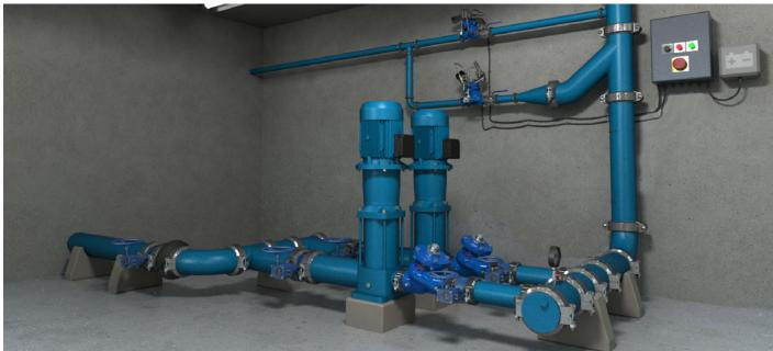
Lift Pump Station with BERMAD BC-80N-P Check Valve preventing reverse flow into the reservoir. The station also features a BC-830-P Pressure Relief Valve that maintains minimal flow if churn operation
