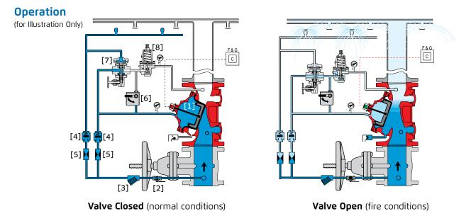
The BERMAD model 400Y-1MC is held closed by water pressure in the control chamber [1]. Upon release of pressure from the control chamber, the valve opens.
