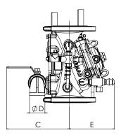
NOTE - The Maximum Allowable Operating Pressure is determined by the selected solenoid valve
