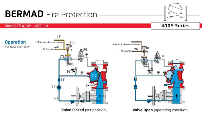
The BERMAD model 400Y-6DC-H is held closed by water pressure in the control chamber [1]. Upon release of pressure from the control chamber, the valve opens.
