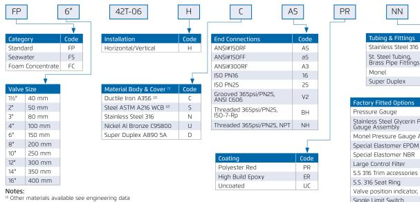
ММ Super Duplex DD Factory Fitted Options Code Pressure Gauge 6 Stainless Steel Glycerin Pressure Gauge Assembly 6п Monel Pressure Gauge Assembly 6m Special Elastomer EPDM F1 Special Elastomer NBR E3 Large Control Filter F S.S 316 Trim accessories Ν S.S. 316 Seat Ring Т Valve position indicator, Linear Single Limit Switch S
