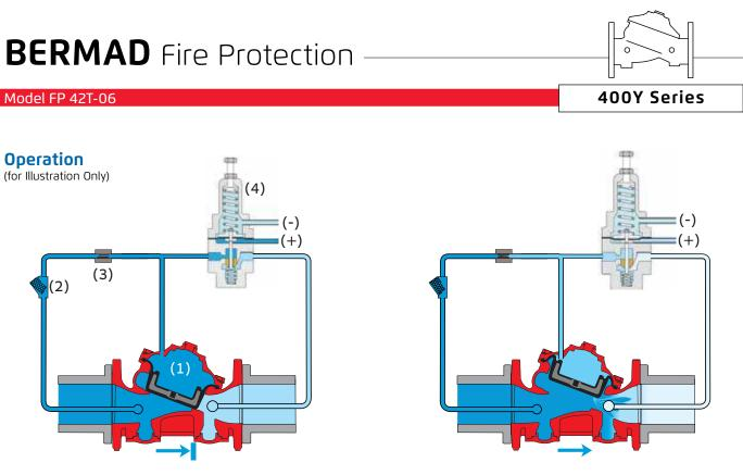
Valve Closed (static condition)
